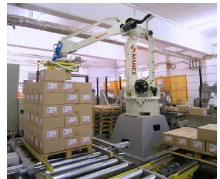
Palletising robot with 2 deposition places
